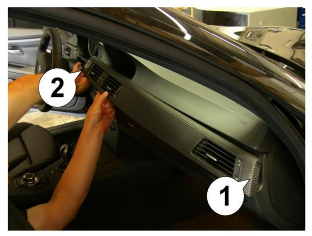
2. Pull out the Climate Control panel and disconnect the plugs on it's back.
