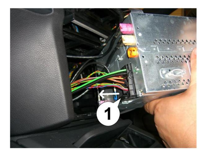
Disconnect CIC unit. Find spitted CAN wires – pins 9 and 11. Cut these wires. Connect emulator like in picture
