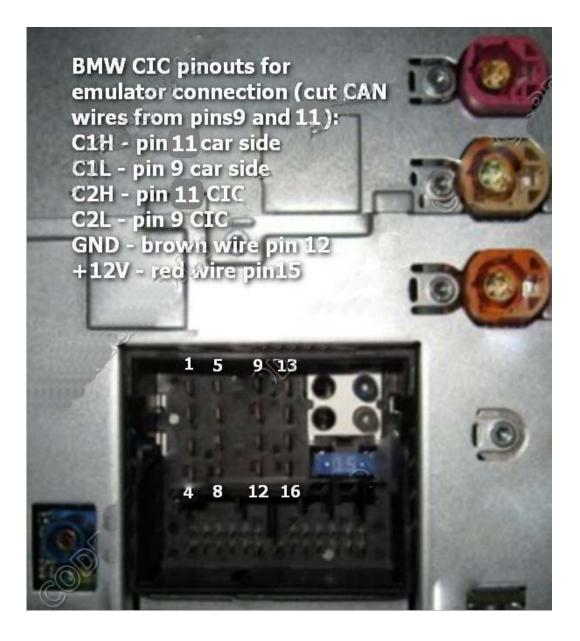
After connection insulate BMW CIC emulator board with heat shrink or insulation tape.
