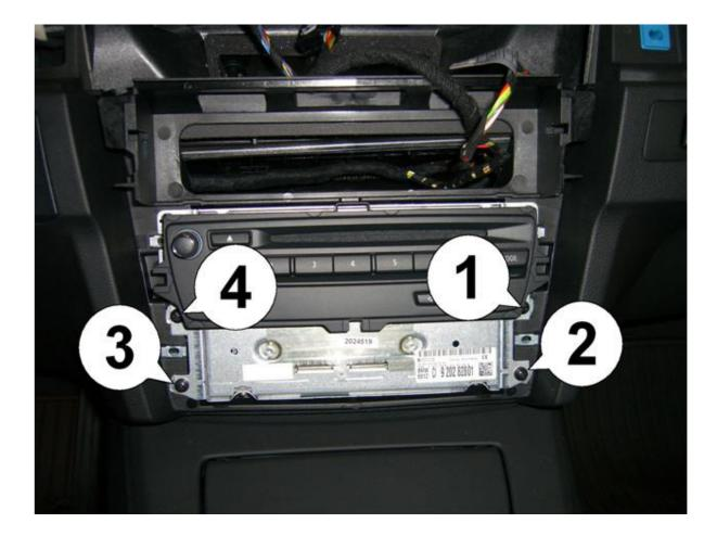
5. Unplug the large black plastic plug by squeezing the tabs (1) together while pulling outward (direction of the arrow).
