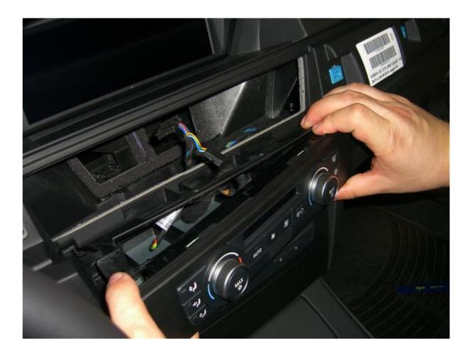
3. Remove cover plate from Multimedia unit keypad. Like all the other parts it is just snapped in place.
